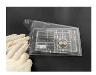
3. Place your finger in the groove of the tray and hold the tapered side of the cartridge and remove the cartridge from the casing.
